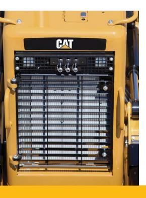
The radiator, air-to-air aftercooler and hydraulic oil cooler are packaged in a single plane, making cleanout easier. Durable, aluminum bar plate construction gives you superior heat transfer and corrosion resistance. 8.9 fins per inch (6.5 fpi on Waste Handlers) on the standard core allow debris to pass through and help reduce plugging.
