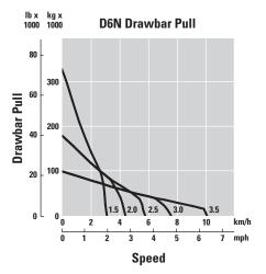
The direct injection electronic fuel system provides a controlled fuel delivery increase as the engine lugs back from rated speed. This results in increased horsepower. A combination of increased torque rise and maximum horsepower improves response, provides greater drawbar pull and faster dozing cycles.
