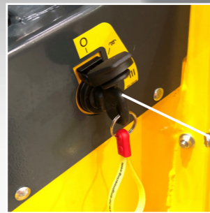
Two stage start inhibitor safety system
